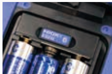
Attach to enable Bluetooth® wireless technology
