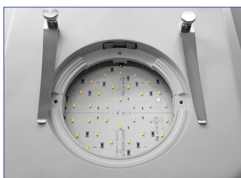
SZ-ST3: 60-Led X-LED 73 Transmitted Illuminator
