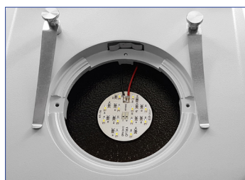
SZ-ST2: 12-Led X-LED 71 Transmitted Illuminator
