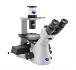
Inverted trinocular LED fluorescence microscope, B & G LED Fluorescence Cubes, IOS LWD W-PLAN PH objectives
