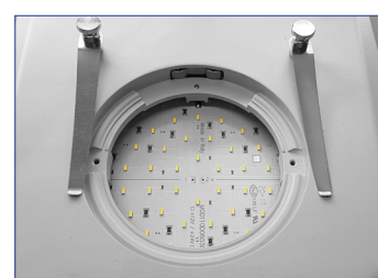
SZ-ST8: 60-Led X-LED 73 Transmitted Illuminator
